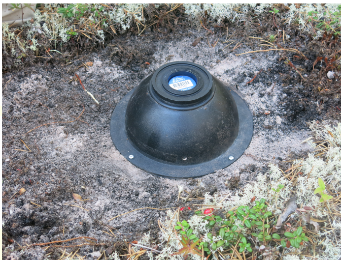
Picture 1 – Radon Flux Monitor in place
